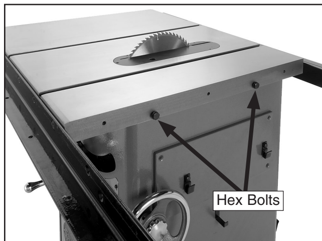
Figure 12. Hex bolts installed.
